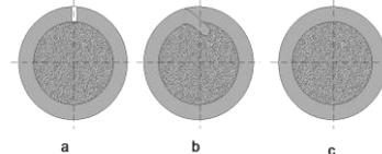
Fig. 1. Closing profile types for tubular electrodes
