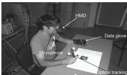
Fig. 2. AR devices used for the interaction and visualisation with the 3D models
