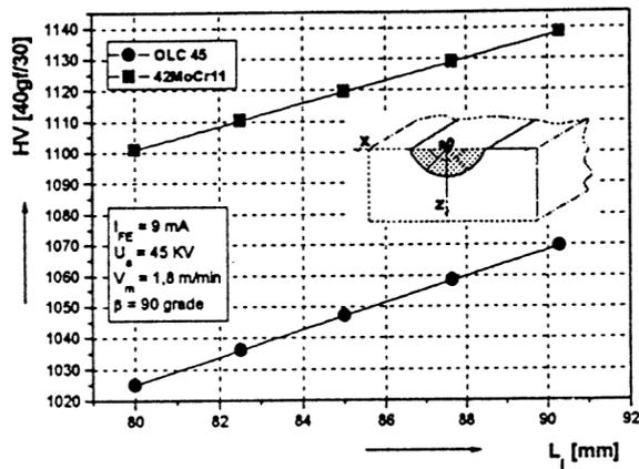
Fig. 3. The effect of the working processing distance  $L_1$  on hardness  $HV$
