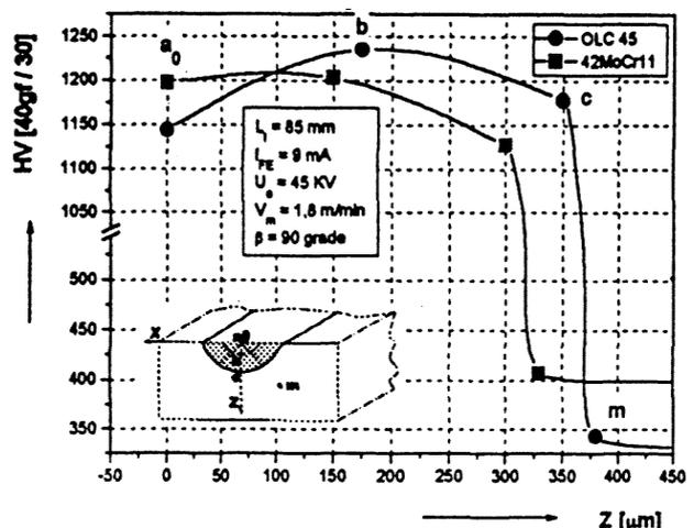
Fig. 2. The depth effect of hardened zone Z on hardness HV
