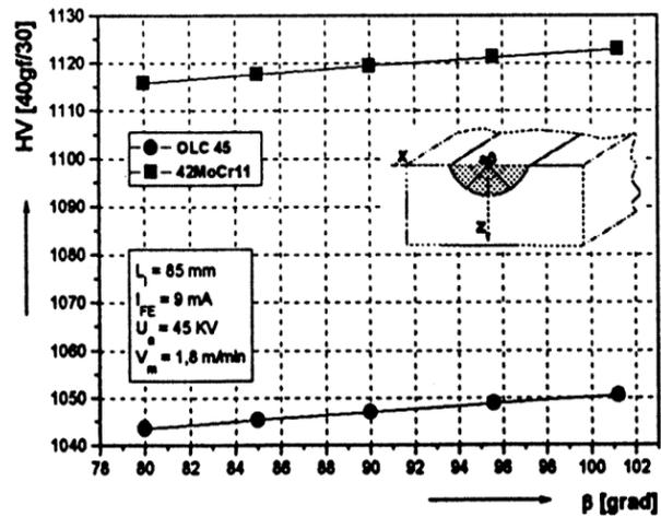
Fig. 5. The effect of cross deflection angle  $\beta$  on hardness  $HV$
