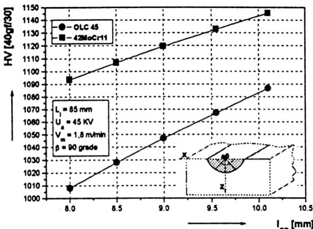
Fig. 4. The effect of electron beam current strength  $I_{FE}$  on hardness  $HV$
