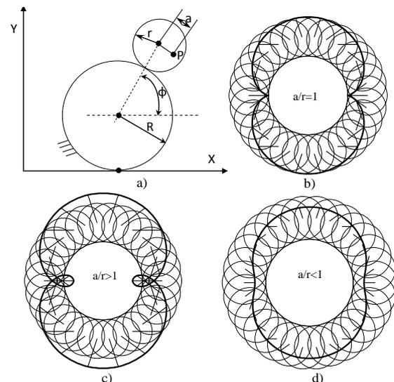
Fig. 2. Epicycloid parameters and different particular cases
