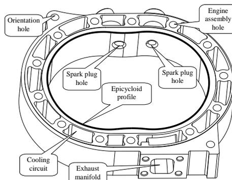
Fig. 1. Wankel housing with epicycloid inside profile
