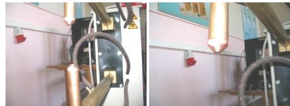
Fig. 2. Contact electrodes mounted on the welding machine
