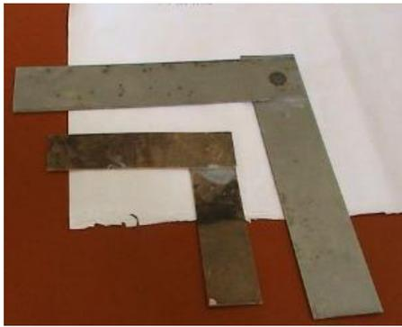
Fig. 4. Comparison between spot welded and brazed samples
