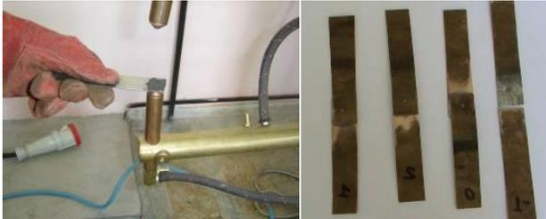
Fig. 5. Making of spot brazed samples from copper plates
