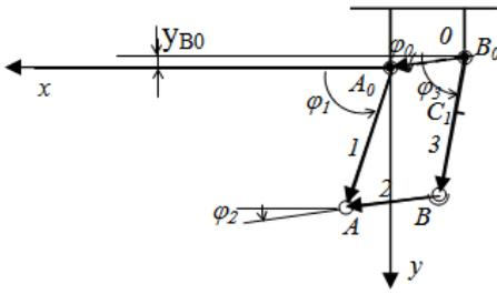
Fig. 3. The vectorial configuration of the first kinematic chain
