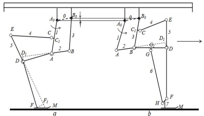
Fig. 2. Kinematical scheme of the mechanisms from posterior legs (a) and anterior (b)
