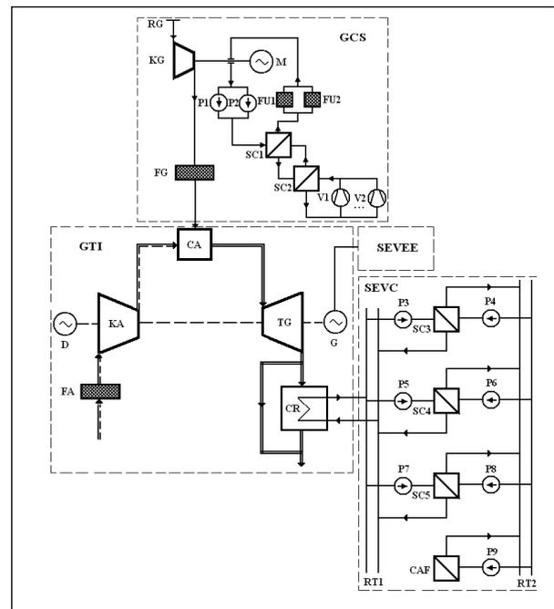
Fig.2. Thermo mechanical scheme of CHP: RG – gas metan network; KG – gas compressor; FG – gas filter; M – engine; P1...P10 – pumps; FU1, FU2 – oil filter; SC1...SC5 – heat exchangers; V1, V2 – air fan; D – starter; FA – air filter; KA – air compressor; CA – combustion chamber; TG – gas turbine; CR – recovery boiler; CAF – hot water boiler; RT1 – heat water collector distribution; RT2 – heating network
