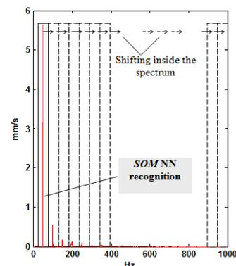
Fig. 1. Operating principle of the SOM neural network for recognizing vibration samples
