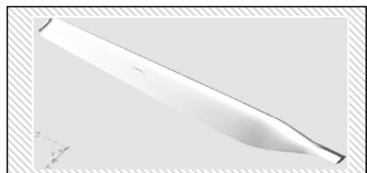
Fig. 1. The blade for wind turbine designed in CATIA program
