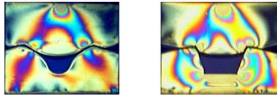
Fig. 5. Izocromates for real profile and new profile at 106 N
