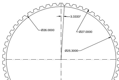
Fig. 1. Geometrical model of the groove roller
