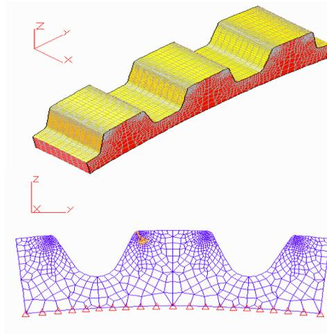
Fig. 2. Model with 3 teeth and 2 cavities
