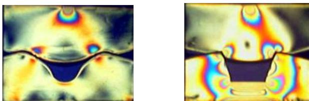
Fig. 4. Izocromates for real profile and new profile at 54,3 N
