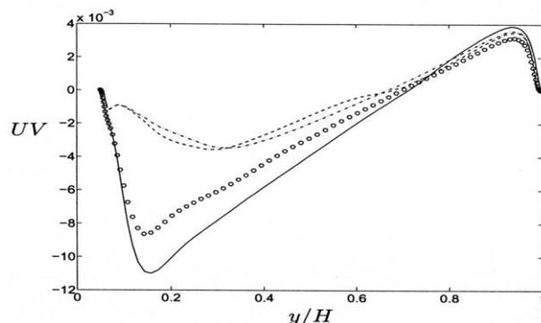
Fig. 1. Comparison of dimensionless Reynolds stress  $UV$  with DNS at location  $x/L = 0$ : (o) DNS of [5], (-) ske model, (-) rke model, (-) rsm model
