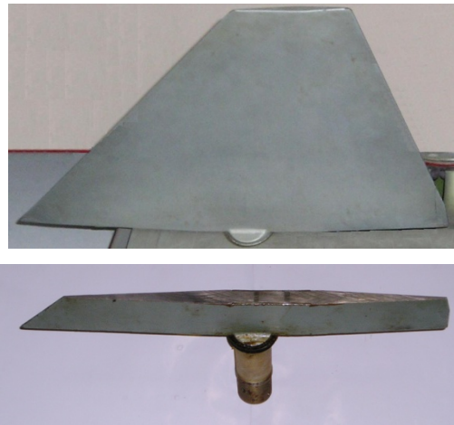
Fig. 2. Aileron in neutral position on fuselage and cut-away
