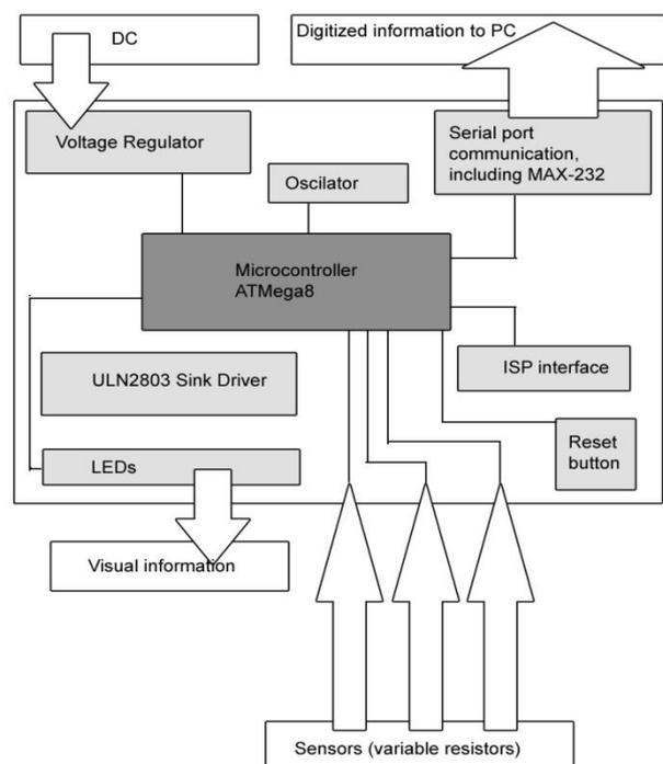
Fig. 1. The PCB with adjustable resistors as sensors
