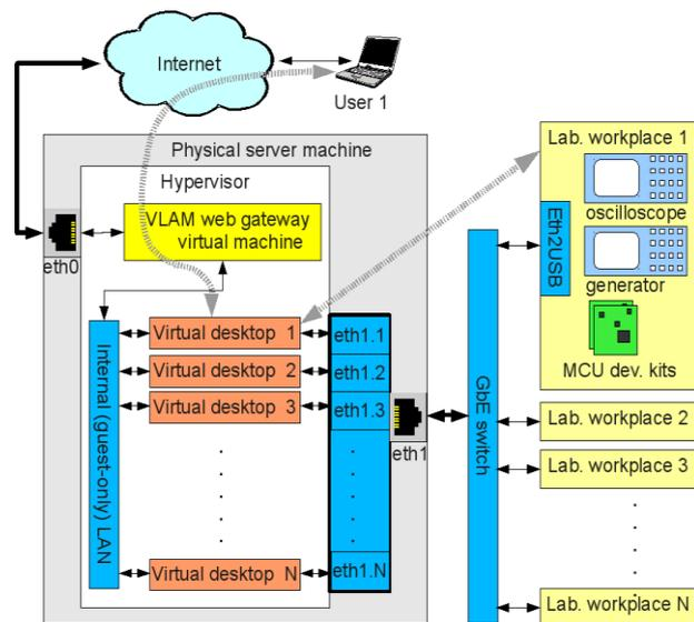
Fig. 1. Basic structure of VLAM system
