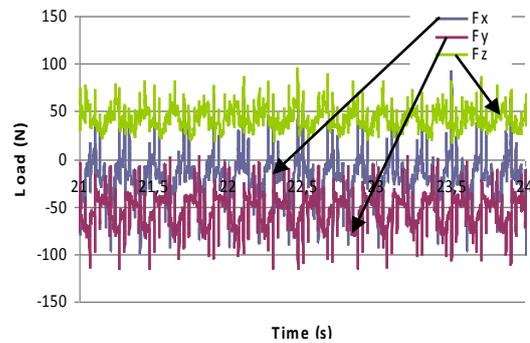
Fig. 4. Experimental resulted cutting forces
