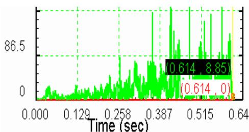
Fig. 3. Predicted cutting force in [N] on Y direction
