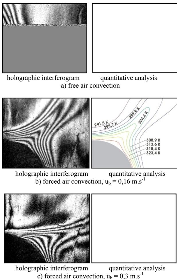
Fig. 1 Temperature fields around the cylinder ( $T_w = 323,5 \text{ K}$ ,  $T_\infty = 291,5 \text{ K}$ ,  $d = 50 \text{ mm}$ ,  $b = 10 \text{ mm}$ )
