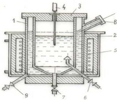
Fig. 2. Electrical heated melting bath for fusible materials
