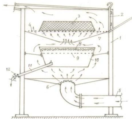
Fig. 3. Filtration device for used moulding compound
