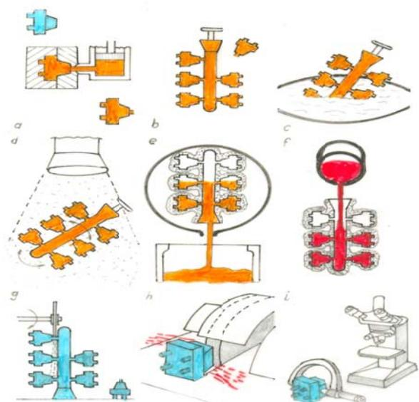
a - models making; b - joining c - lodging of refractory paint; d – fixation of refractory material, e - removing of the fusible models from the moulding shell, f – casting the alloy, g – removing the parts from the cluster; h - cleaning and finishing the parts, i – quality control of the final product.
