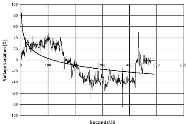
Fig.5. Recorded time delay minimize nuisance tripping due to grid system disturbances
