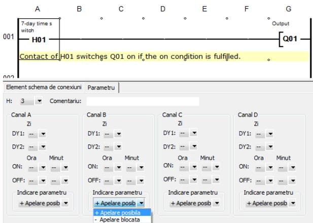
Fig.4. Line sequence for coding Easy 500 Relay in order to fulfil main program requirements
