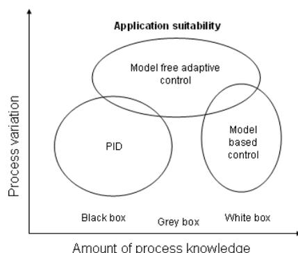
Fig.1. Application suitability from process validation point of view, correlated with the process knowledge
