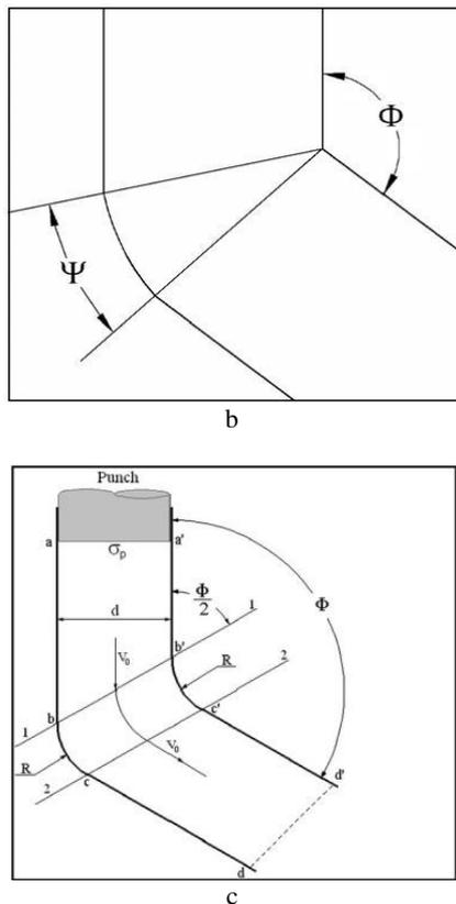
Fig. 1. Segal's geometry (a), Iwahashi's geometry (b) and Luis' geometry (c)
