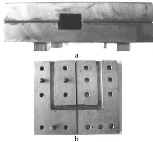
Fig. 2. ECAE die: profile (a) and the two parts that make the die body (b)
