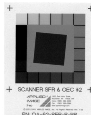
Fig. 1. Quality Assurance 62 sharpness calibration target
