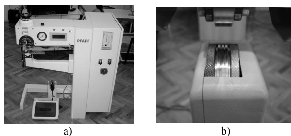
Fig. 1. Ultrasonic welding equipment, a) Seamsonic 8310-003, b) Anvil wheel
