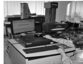
Fig. 1. Nanometric equipment for the control of micro-roughness and of the micro-contour of surface
