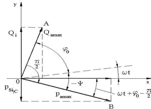
Fig. 2 The vector graphic to the sonic pressure and the sonic flow
