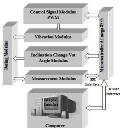
Fig. 2. Block chart of automatic dosing system
