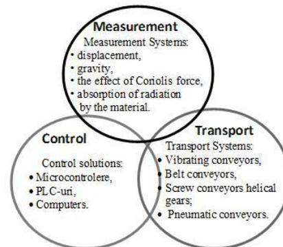
Fig. 1. Dosing system requirements
