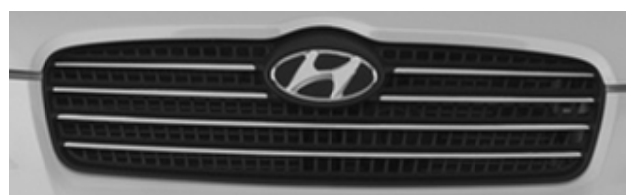
Fig. 2. A front radiator grill with chrome-plated film inserts made by FIM method
