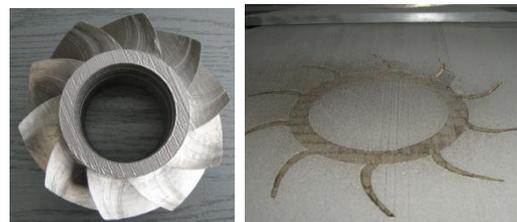
Fig. 3. SLM process, stainless steel
