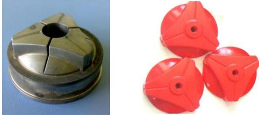
Fig. 4. Injection molded parts, using the SLS tools
