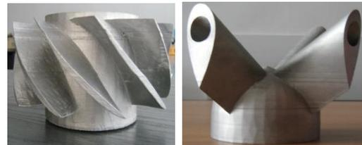
Fig. 2. Complex steel parts, made by SLM at TUCN
