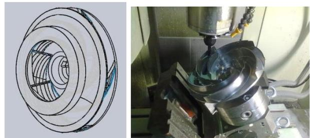
Fig. 5. Complex product - stainless steel, CNC milling
