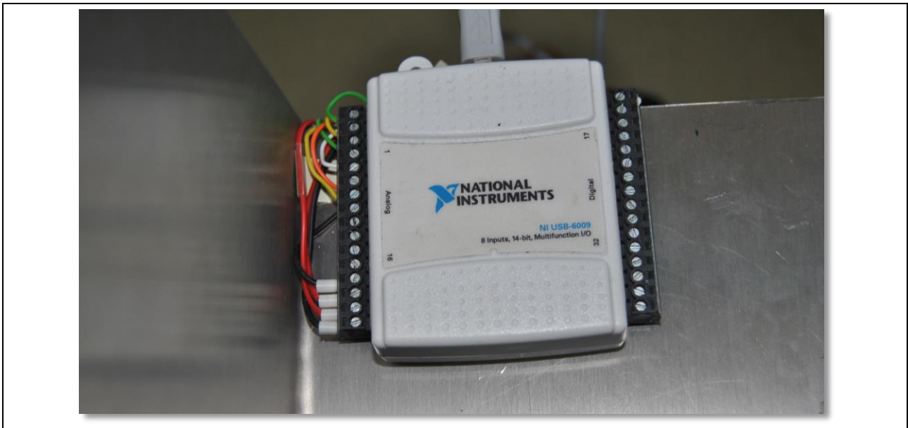
Fig. 3. NI USB-6009 controller card used to control the servomotors
