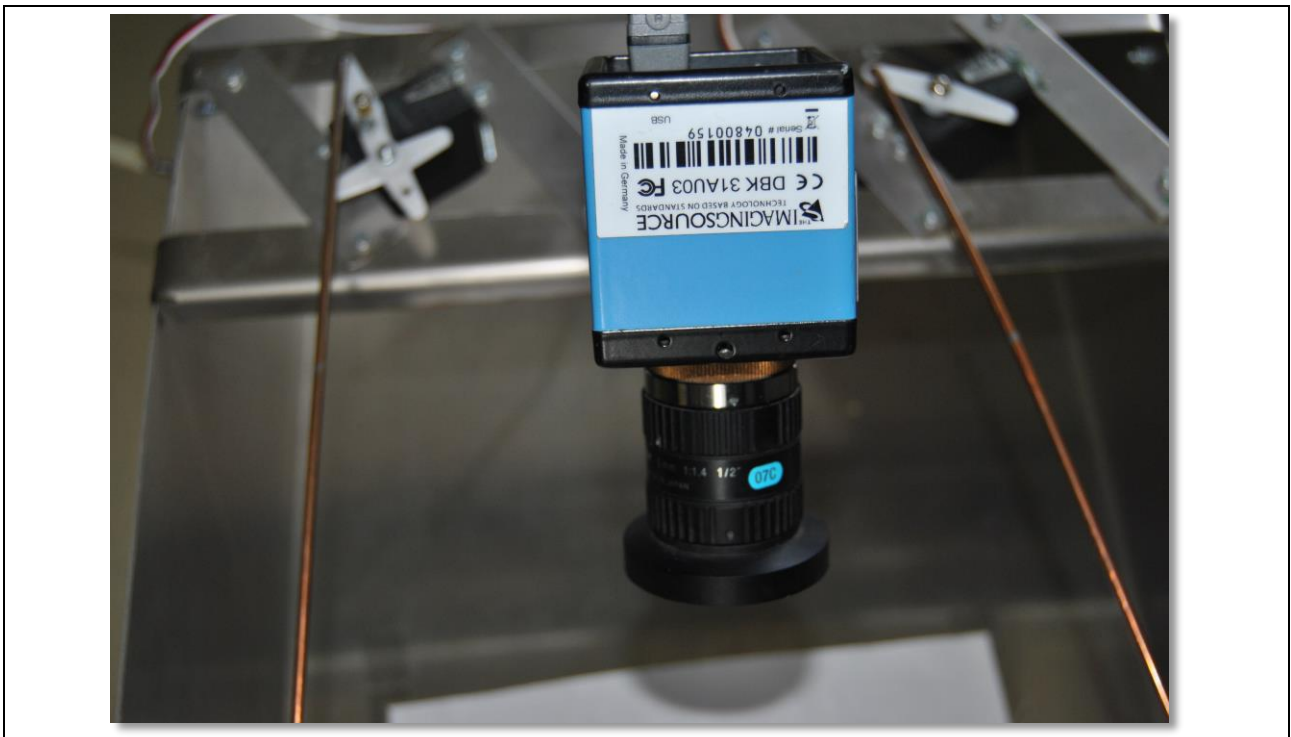
Fig. 2. The imaging source's DBK31AU03.AS digital camera used to capture new images on the sorting line
