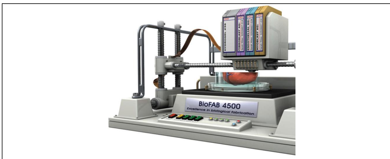
Fig. 2. A conceptual model of an organ printer (Tarik Ozbolat, 2013)
