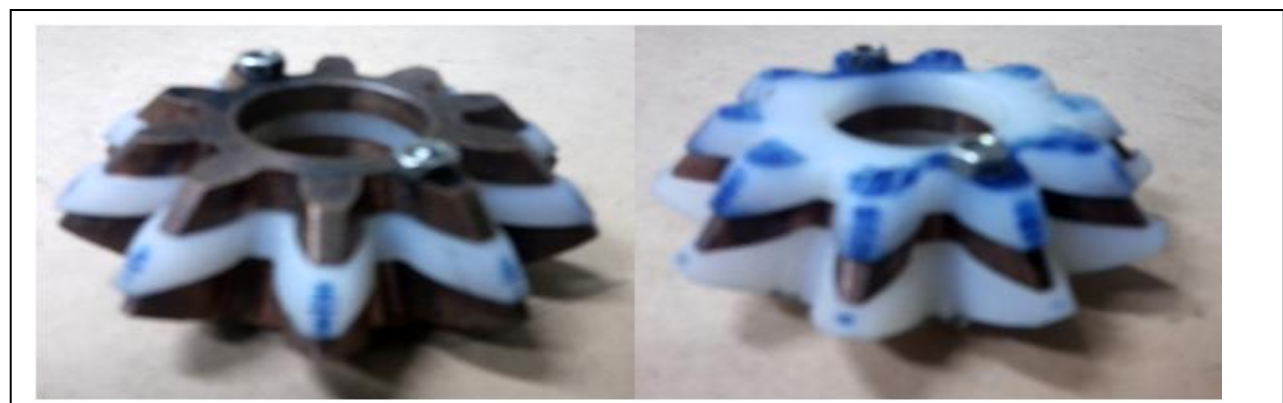
Fig. 2. Complementary cathode gears used for finishing the bevel gears by ECH
