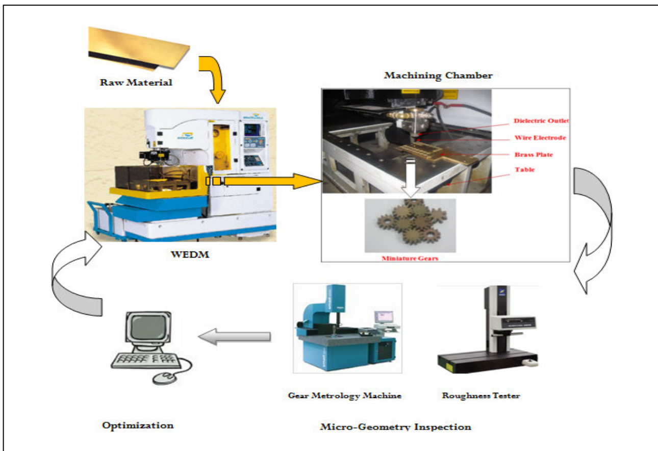
Fig. 3. Process sequence for manufacturing of miniature gears by WEDM
