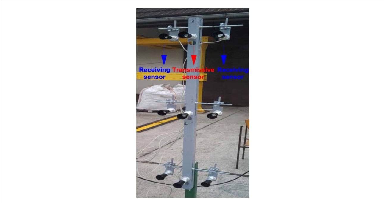
Fig. 2. The distribution of sensors; the middle three sensors generate an ultrasonic burst, while the left and right group receives it
