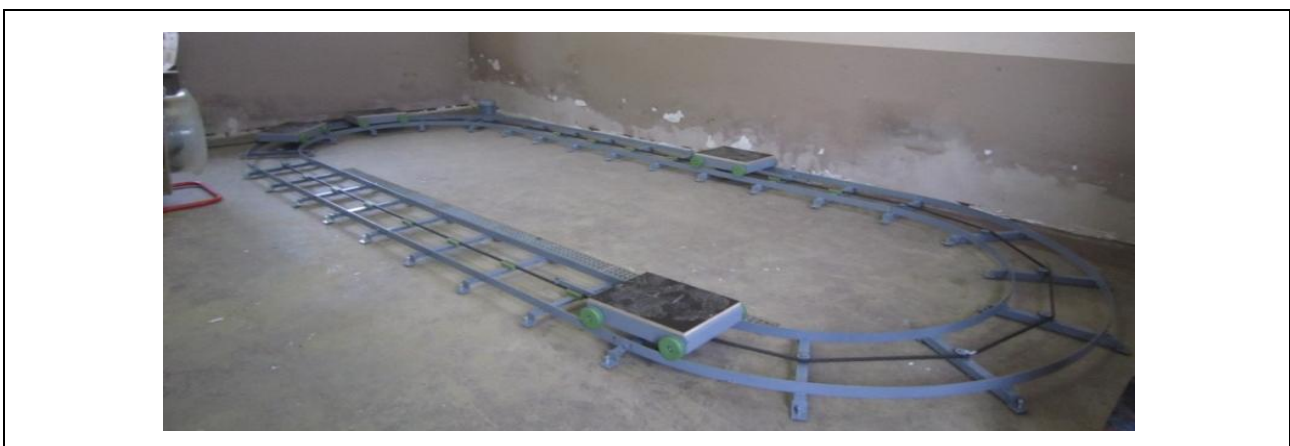
Fig. 3. Composite track for testing ultrasonic measurement system
