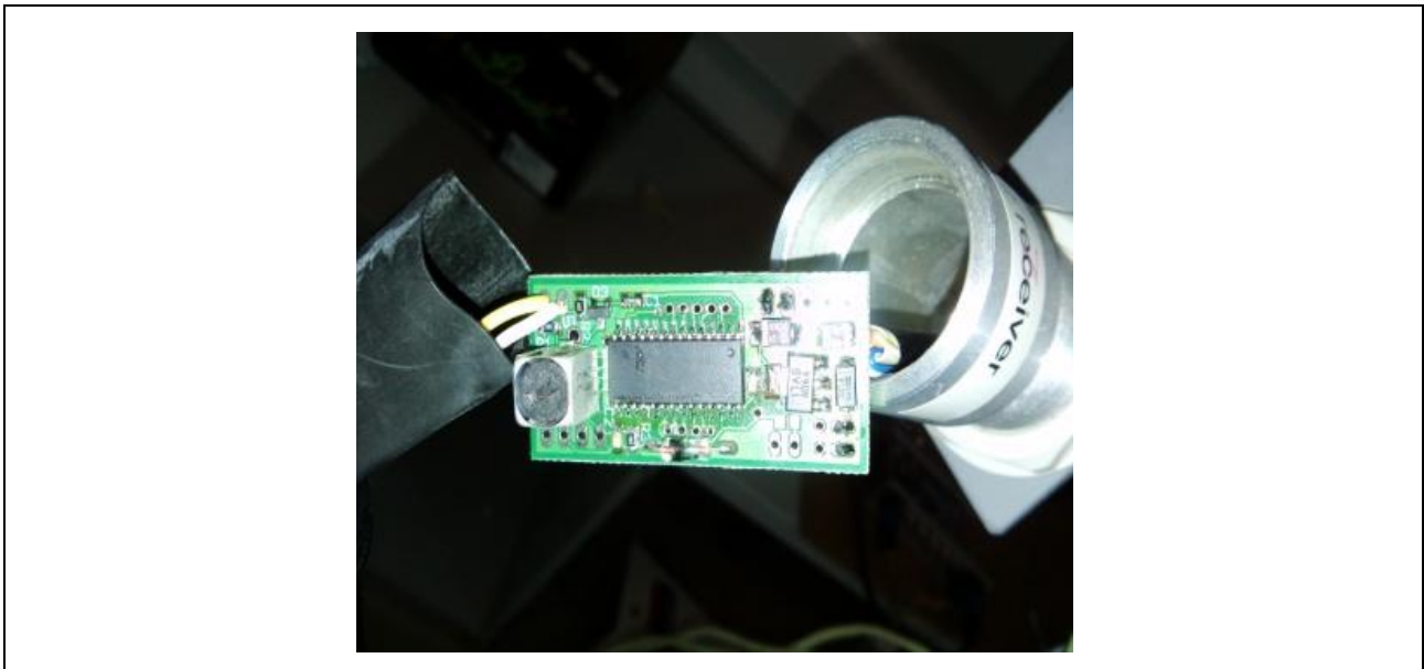
Fig. 1. The sensor circuit build around a PROWAVE 400EP250 transmitter and CYPRESS CY8C29466-24SXI FPGA microcontroller
