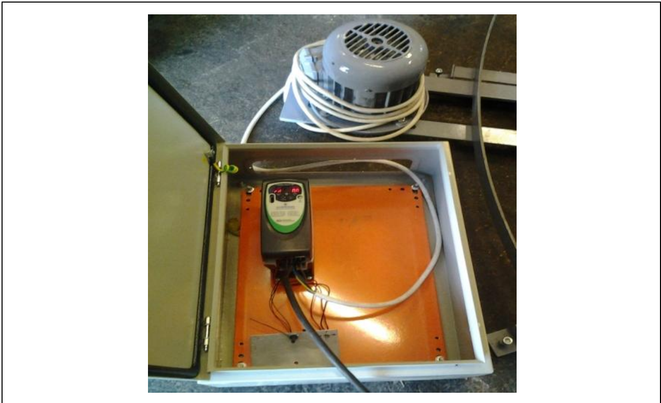
Fig. 4. Universal open-loop 3-phase frequency regulator that was used to fine-tune the traveling speeds
