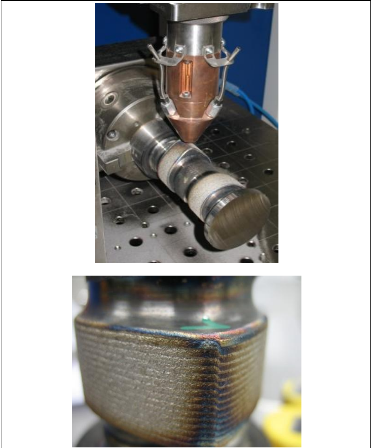
Fig. 8. Laser cladding of camshafts. Courtesy of TRUMPF
