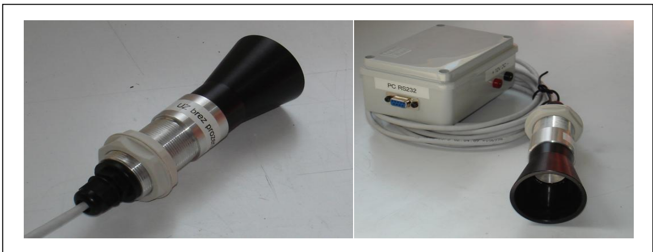
Fig. 3. Ultrasonic sensor with ultrasonic transceiver built in the horn. The enclosure includes sensor electronics (Jejčič et al. 2011).
