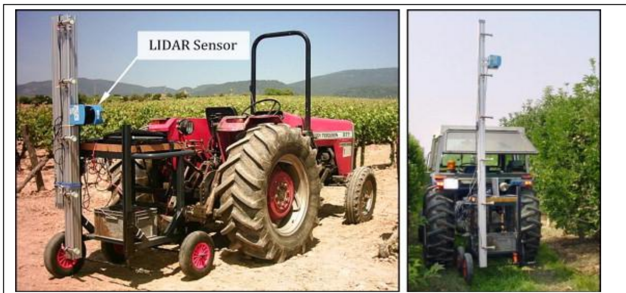
Fig. 1. LIDAR 3D dynamic measurement system (Rosell & Sanz, 2012)
