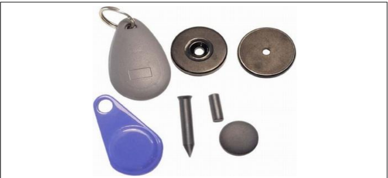
Fig. 2. Various forms of RFID tags (Stankovski et al., 2010)
