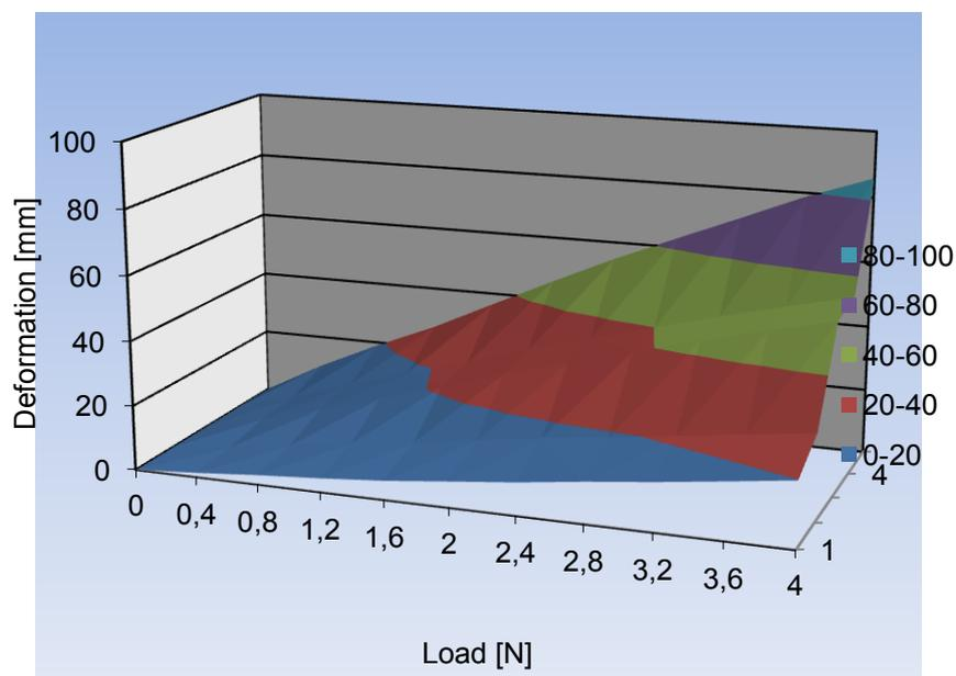
Fig. 4. Dependence of deflection under load for the set of uncoated state wires
