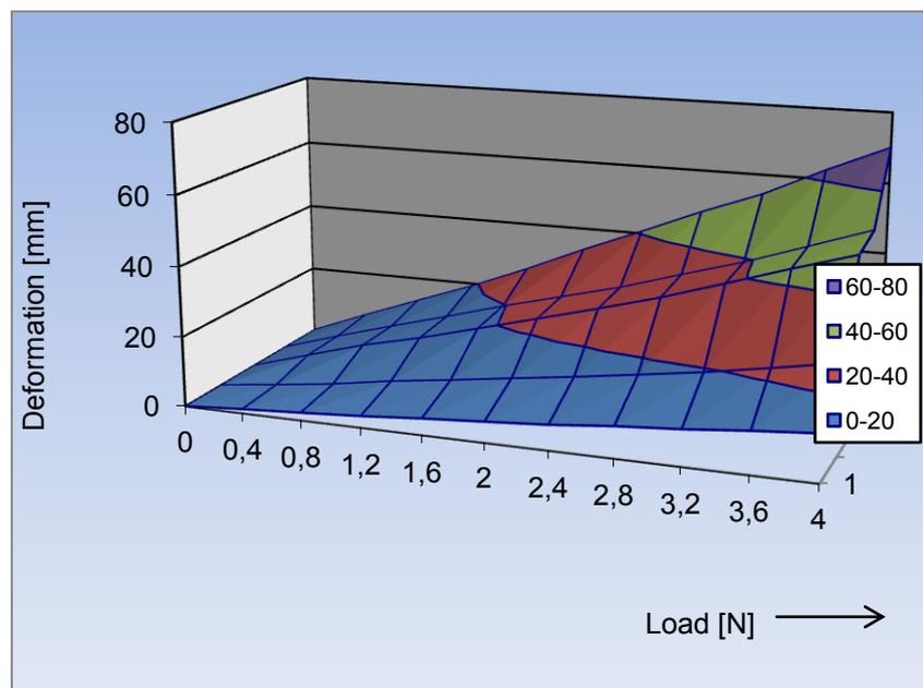
Fig. 6. Dependence of deflection under load for the set (a) of uncoated state wires
