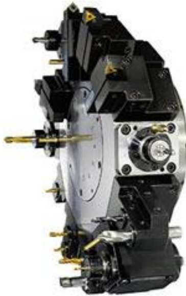
Fig. 1. Turret with turning and rotary tools
