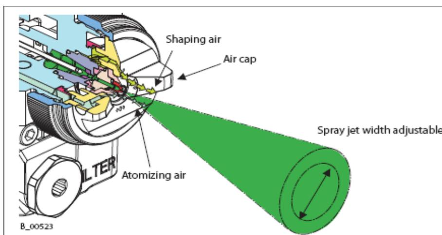
Fig. 3. The principle of hydrodynamic spraying (\*\*\*, 2010)
