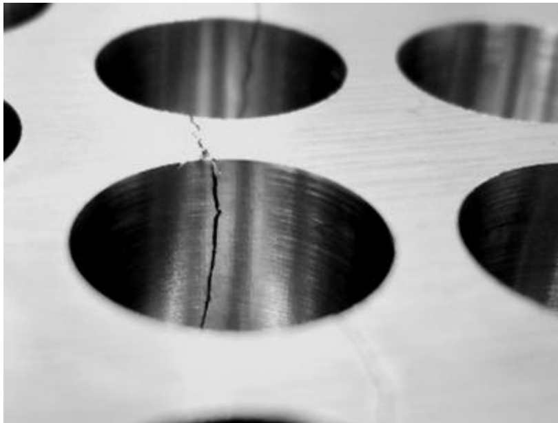
Fig. 9. Fragile fracture during BHM process on TNB alloy
