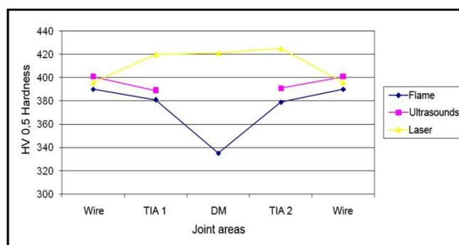
Fig. 7. Evolution of hardness in wire – wire joint areas
