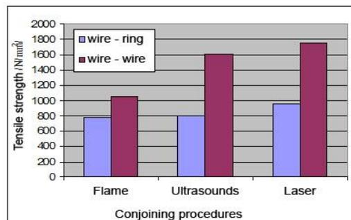
Fig. 4. Tensile strength of welded joints
