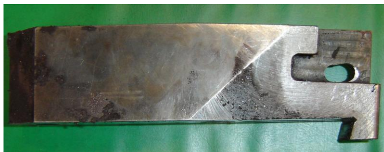
Fig. 2. Standard tool used on wheel-turning lathe
