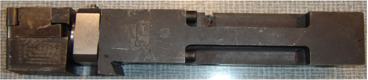
Fig. 3. Special tool with inserted force meter
