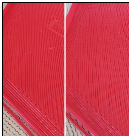
Fig. 16. Printing lines difference (left: 15 1/min, right: 25 1/min)
