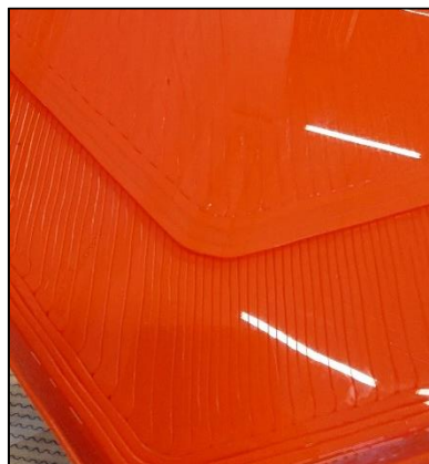
Fig. 14. Surface between object and print bed (top: with bed leveling system, bottom: without bed leveling system)
