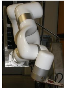
Fig. 4 - Methodology validation results. Beginning state is given in E) roll angle 0 deg and pitch angle 15 deg, G) roll angle 0 deg and pitch angle 0 deg and ending state is given in F). In frames from the left to right xArm base mounting orientation from xArm control GUI, front and side view of actual manipulator state, IMU data visualization razor_imu_9dof razor-pub-and-display.launch.
