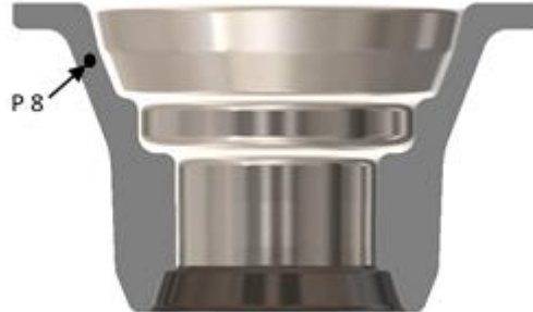
Fig. 1. General view of the forged part, a cross-section with the point selected for modelling, and its total true strain level
