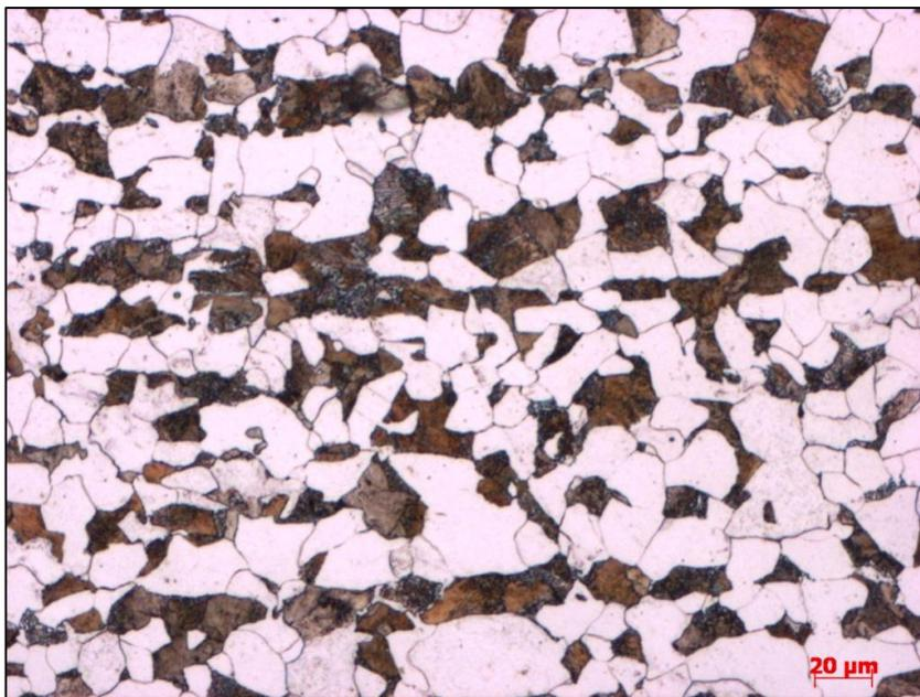
Fig. 1. Microstructure of base metal - steel E295.
