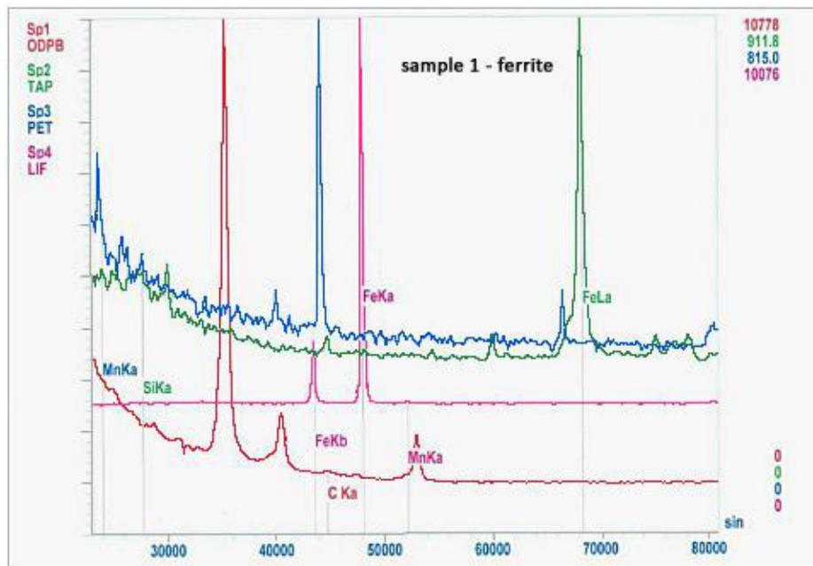
Fig. 5. Example of qualitative spectral analysis on Sample 1.
