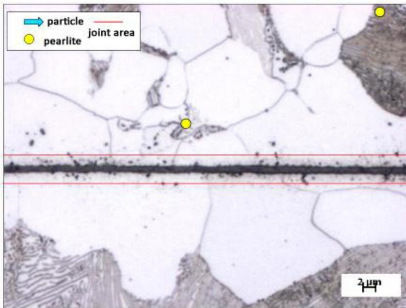
Fig. 4. Microstructure of sample 3:  $T = 1\ 000^{\circ}\text{C}$ ;  $t_s = 900\ \text{s}$ .
