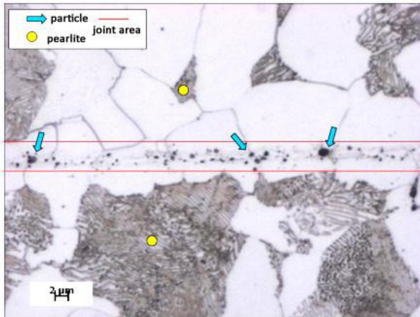
Fig. 3. Microstructure of sample 2:  $T = 1\ 000^{\circ}\text{C}$ ;  $t_s = 600\ \text{s}$ .
