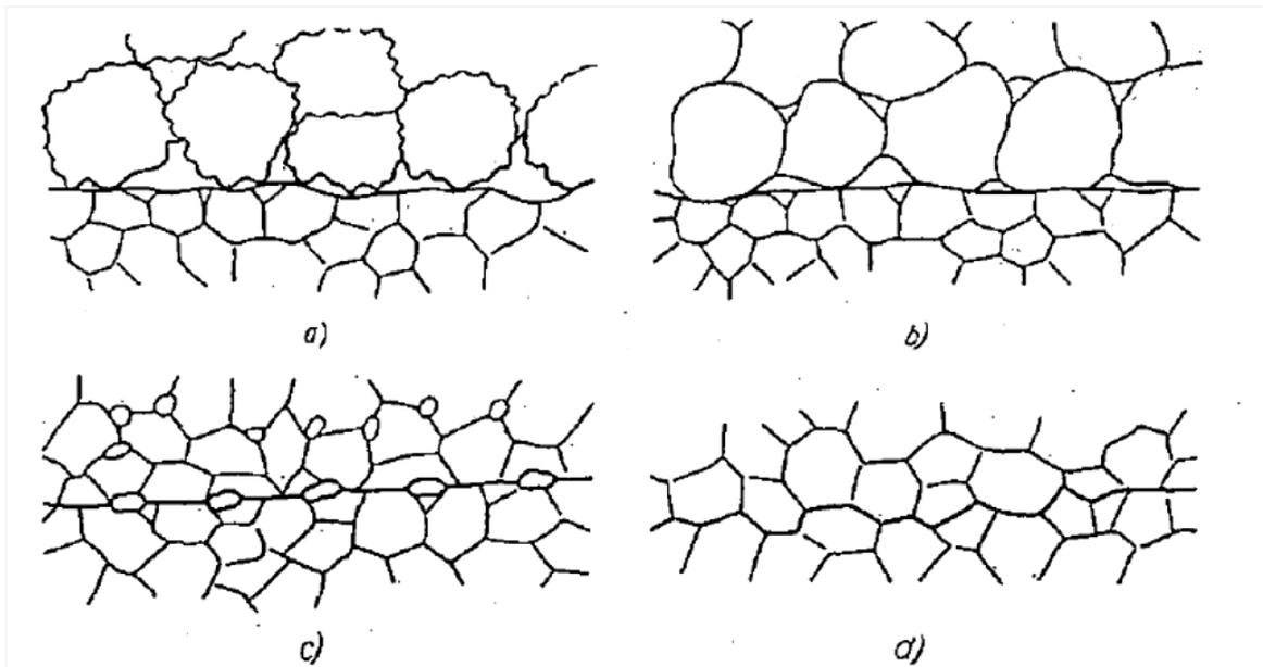
Fig. 6. Stages of creating diffusion joint [3], (a) The first contact, migration of atoms and bridges creation, (b) The plastic alignment of micro-roughness, (c) The intensive diffusion and micro-deformation, (d) The ideal diffusion joint.
