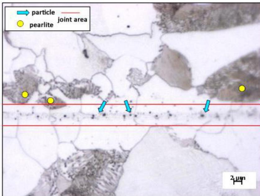
Fig. 2. Microstructure of sample 1: T = 1 000°C;  $t_s$  = 300 s.
