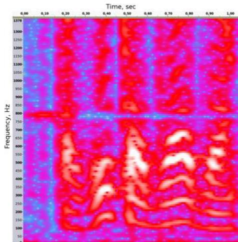
Fig. 1. Howling detected at the frequency of 790 kHz in the first frame and then filtrated with the narrow band notch filter.
