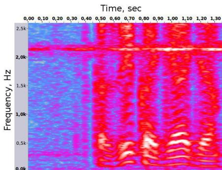
Fig. 2. Unpleasant effect – howling at the frequency about 2.2 kHz.
