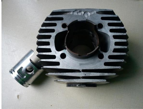
Fig. 10. The finished cylinder.
