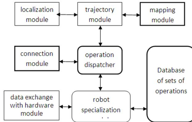
Fig. 1. The software structure.
