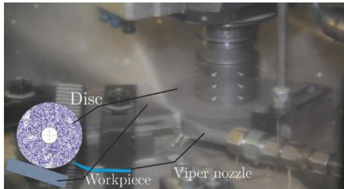
Fig. 4. ViperCut© nozzle with process illustration.
