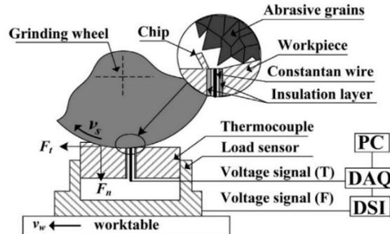
Fig. 3. Sketch of measurement system (DSI: dynamic strain indicator, DAQ: data acquisition card, T: temperature, F: force) [6].
