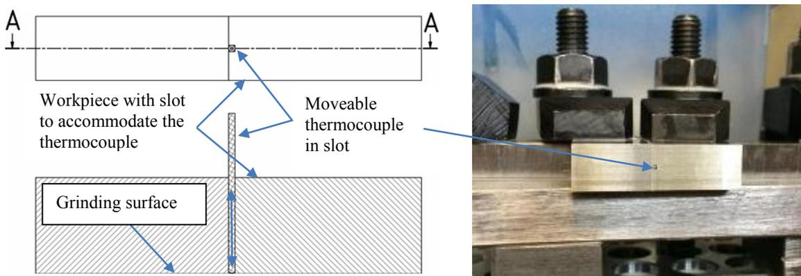
Fig. 5. Experiment setup with cross-section of the workpiece and thermocouple in the slot; left and mounted on the machine; right.
