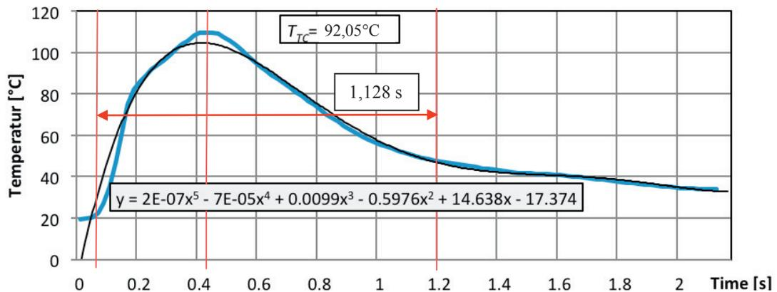
Fig. 7. Temperature curve of the thermocouple during up-cut grinding with a mean temperature of  $\Delta T_{TC,mean}=58^{\circ}\text{C}$  for the contact length of 44,3 mm and  $t_{el}=1,128$  s.
