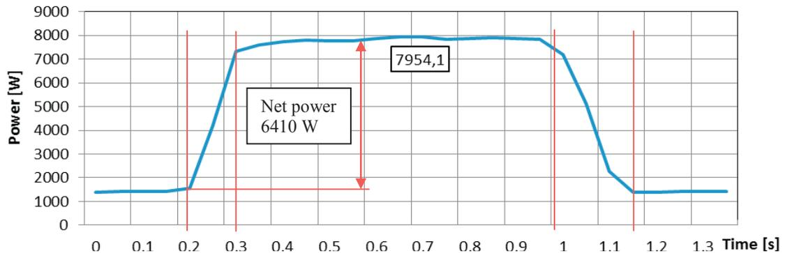
Fig. 6. Power curve of the spindle during the climb grinding operation.
