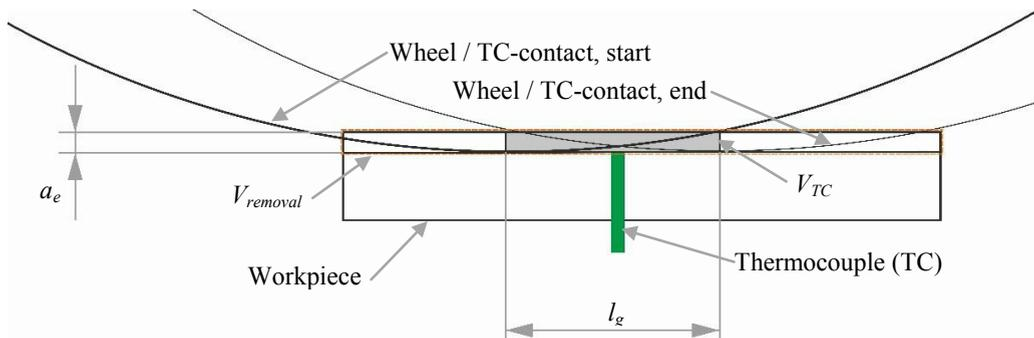
Fig. 8. The geometrical contact length  $l_g$  accounts for the distance when the wheel moves past the thermocouple.
