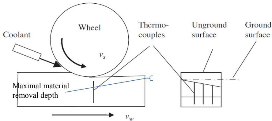
Fig. 1. Temperature measuring in the grinding zone with a thermocouple in a small hole and indication of the maximal material removal depth [1].
