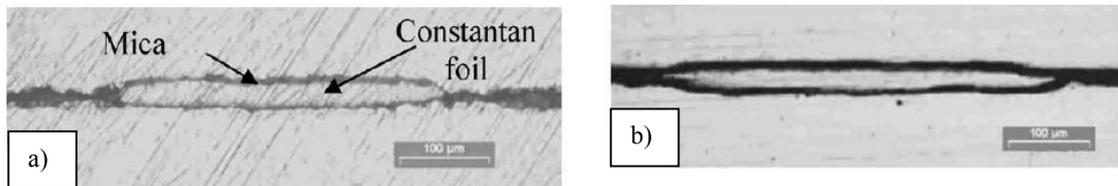
Fig. 2. Close up of the arrangement of the constantan foil and mica film before grinding (a) and after grinding (b) [3].
