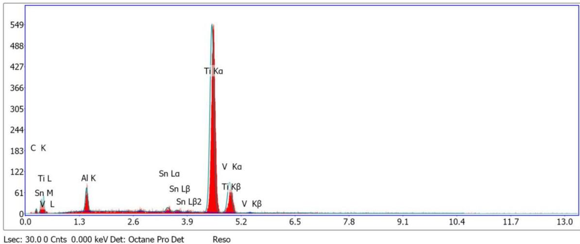
Fig. 3. Ti 6Al 4V composition data by EDX analysis.
