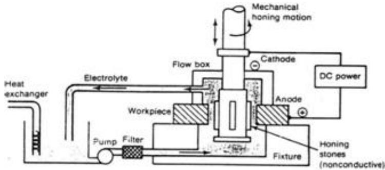
Fig. 1. Schematic view of ECH tool with Work piece Interaction.
