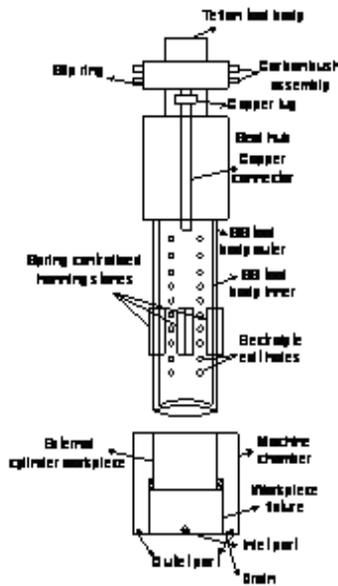
Fig. 2. Exploded view of ECH tool with Work piece fixture.
