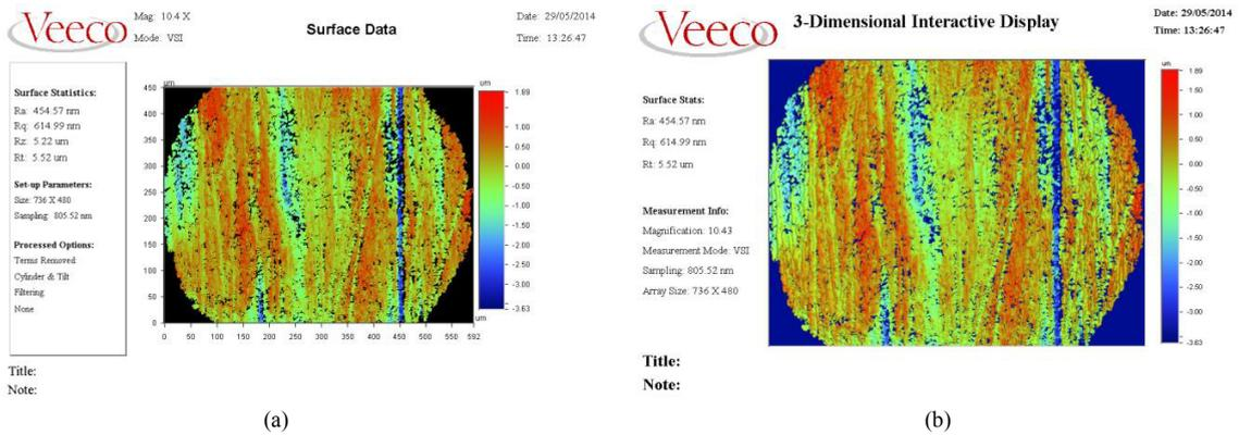
Fig. 4. (a) Average surface roughness data; (b) Average surface roughness 3D interactive data.
