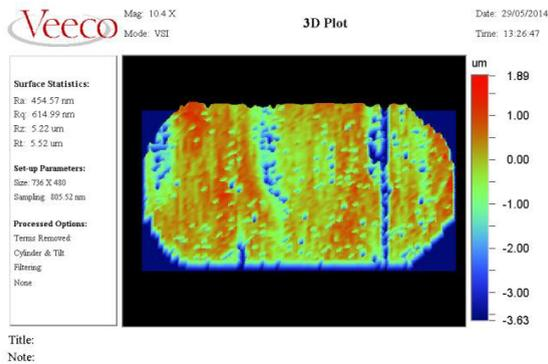
Fig. 5. Average surface roughness 3D plot data.
