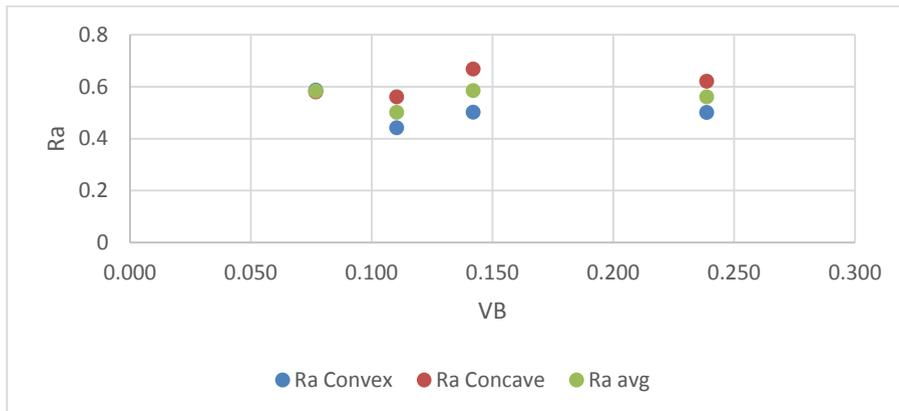
Fig. 9. Correlation between tool wear and average roughness.
