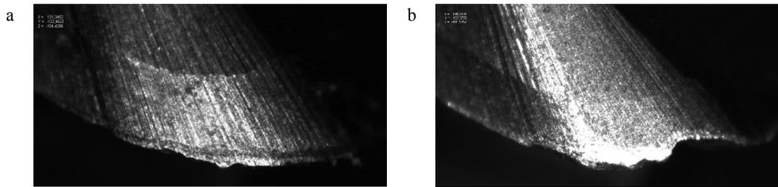
Fig. 10. (a) Cutting tool after Inconel 718 conventional machining (b) Cutting tool after Inconel 738 LC conventional machining.
