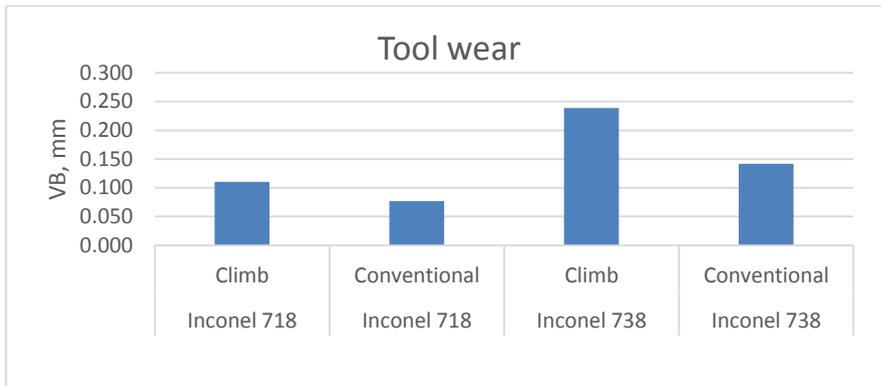
Fig. 8. Tools wear measured values (VB).
